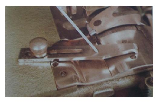
4. Pressure foot: This holds the material to the cutting knife and determines the amount of material to be cut off.
