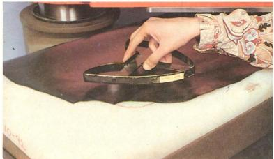
15. Adjust the pressure stroke height, if required, this should be a minimum of 10mm above the knife and no more than 15mm.
