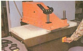
2. Set the arm stroke. Place the knife on the clicking board.
