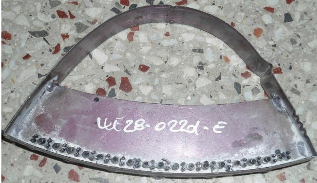
Counter knife: This knife cuts counter part of a shoe. The counter is divided up into three main quality regions.
